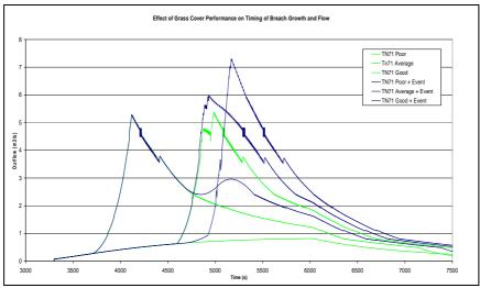
Figure 3. Example of the effect on breach prediction of initiation timing
