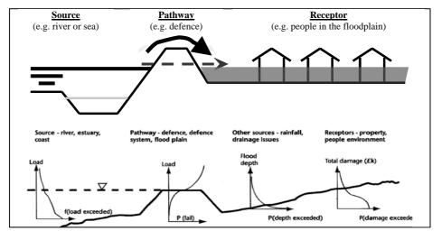
Figure 4. The source-pathway-receptor-consequences model for flood risk (Sayers et al., 2002)
